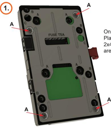
On the back of the UNIX Plate, locate the 4 screws 2x4mm (On illustration they are marked as letter A).
