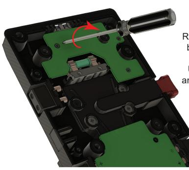
Return the internal USB PCB back to the original position.
