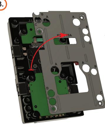
Remove the metal back plate from the UNIX body.
